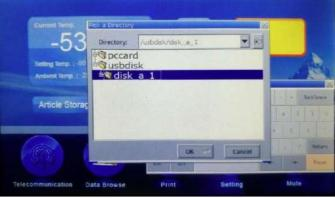
2.reading the data: Connect the U disk to computer, find:\history\datalog\001 as shown as following:
