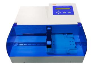
Elisa microplate washer, with 8 or 12 washing probes suitable with 96-well and 48-well microplates.
