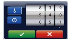
The simple conversational graphic user interface, which has intuitive spinning wheels, makes adjustment of experiment temperature, time and cycle easy.
