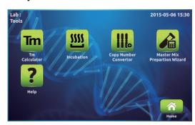
The sensitive 7" capacitive touchscreen enables easy operation even with laboratory gloves on.
